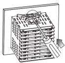
Mount the product on the panel, fasten bracket by pushing with tools as shown above.
