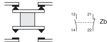
The 2 moving contacts are electrically separated
