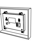
Step 4: For heat dissipation, keep a minimum clearance of 60 mm (2.36 inches) and 45 mm (1.77 inches) respectively on the rear and bottom of the HMI.
