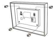
Tighten the screws with the torque less than 0.5 N-M / 0.7 N-M to avoid damage to the plastic clearance of 60 mm on the rear of the HMI.
