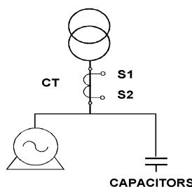
The current transformer, CT, must be located so that it measures the whole load current plus the correction capacitors
