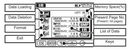
Functions to recall (⇒displays the saved data), delete (⇒deletes the saved data) and format the data (⇒formats the internal memory) are available. Details of each parameter are as follows.
