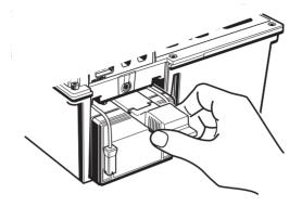
⑤ Pull up the Battery Connectors upward as indicated by arrow mark in the below left illustration, and remove them.
