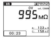
10 This instrument has an auto-discharge function. With the test leads connected to the circuit under test, release the Test button to discharge capacitance in the circuit after test.
