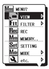
Move the cursor with the UP/DOWN Keys or Shuttle Switch, and confirm the selection with the ENTER Key. Pressing the ESC Key while the Menu is being displayed closes the Menu Window. Items displayed with "" mark are accompanied with submenus. Press the ENTER Key to access to the submenus.
