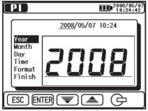
Select " Clock Setting on the ENTER Menu (=>P.37). Adjust the time in a following order: [year], [month], [day], [hour], [minute] and [display format]. Pressing the ENTER Key confirms the entry and proceeds to next step. Press the ESC Key to return to the previous item.
