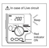
$\begin{picture}(100,0) \put(0,0){\line(0,0){100}} \put(0,0){\line(0,0){10$ displayed, buzzer sounds, and the ALARM indicator lights up. In this case, the test voltage cannot be output by pressing the MEASURE or LOCK button. Disconnect the power supply from the object to be measured and try again.
