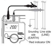
ACV and DCV are automatically detected
